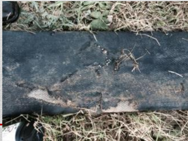
Flaking from UV exposure
